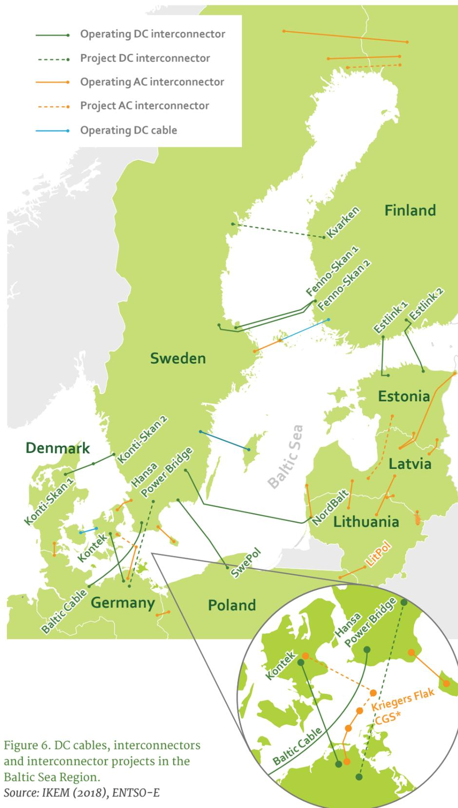
Figure 6. DC cables, interconnectors and interconnector projects in the Baltic Sea Region.
